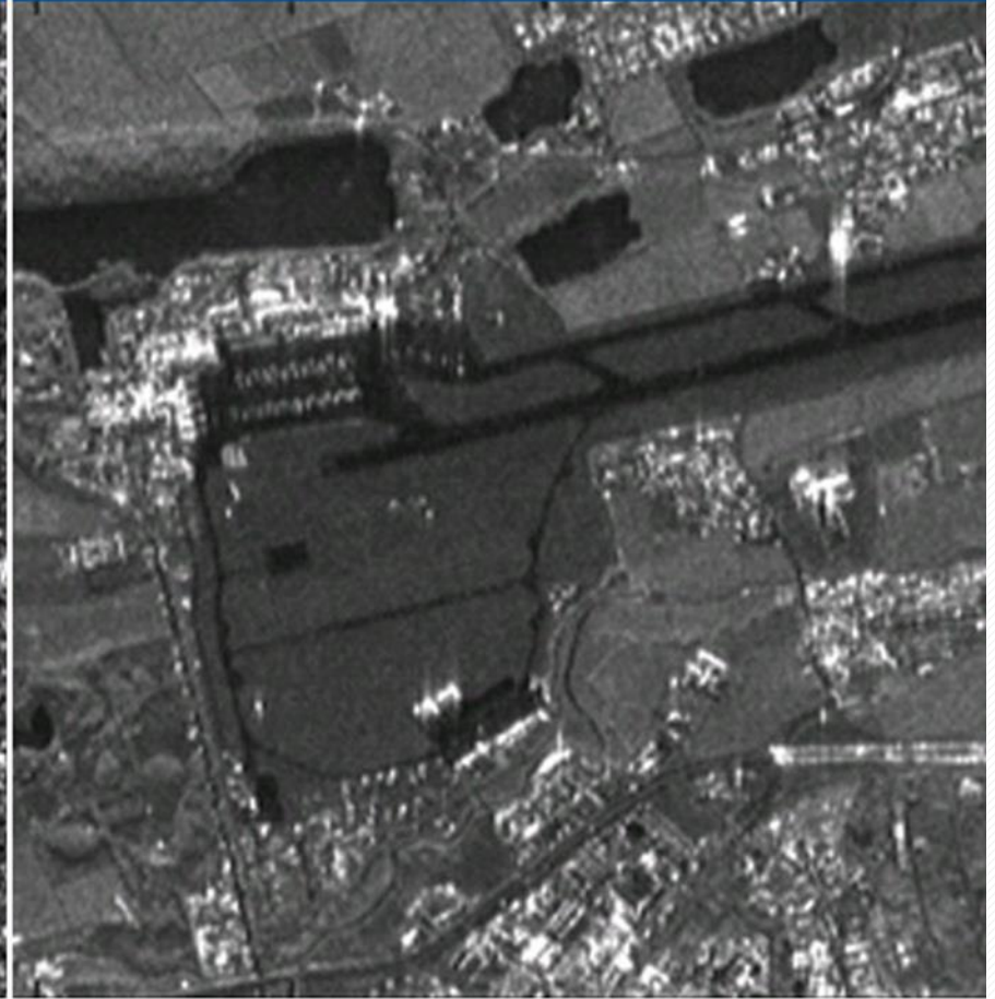
SAR signal amplitude and MIR (Multi Image Reflectivity) map
