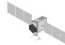
GLONASS 3 Orbital planes 21 Satellites + 3 spares 64.8° Inclination angle Altitude 19,100 km
