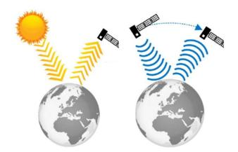
Passive instruments can measure energy that is naturally available. The sun's energy is either reflected, as it is for visible wavelengths, or absorbed and then re-emitted, as it is for thermal infrared wavelengths; due to these wavelengts, in general, passive satellites are not able to work during the night or through the clouds. Examples of passive satellite Earth Observation missions are: MODIS, Landsat-8, Worldview-4, Pleiades, Sentinel-2.
